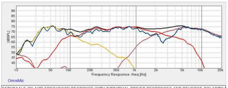
ENTHRAALS ON AXIS FREQUENCY RESPONSE WITH INIDIVIDUAL DRIVER RESPONSES AND REVERSE POLARITY I
