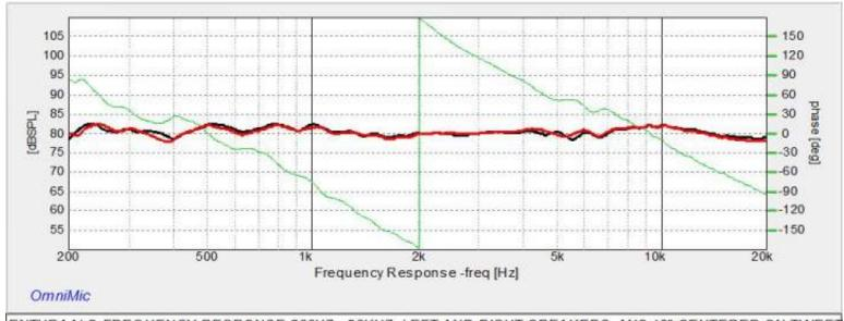
ENTHRAALS FREQUENCY RESPONSE 200HZ - 20KHZ, LEFT AND RIGHT SPEAKERS, MIC 18" CENTERED ON TWEET
