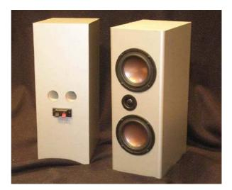
The enclosure could be lined with convoluted foam, which is pretty standard for a vented design such as this. In my case, to keep things simple, I did not line the enclosure at all. Instead, I used a few light handfuls of polyfil behind the woofers (the internal braces sort of held it in place). As I told many people who built the original Overnight Sensations,
